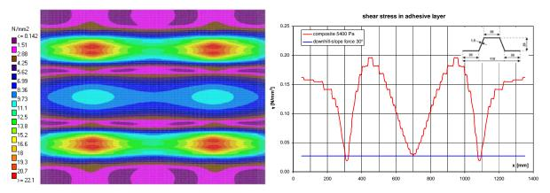
Fig 5 Stresses with backrails (1400x1100x7,0)
